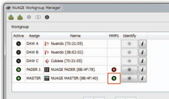
When the MMP1 indicator lights up in red (this means connection failure), the possible causes are as follows:
