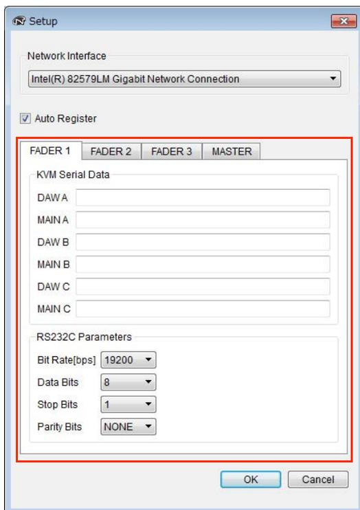
In the DAW A field, for example, you should enter the ASCII message to be sent to the KVM switches to switch them to DAW A when the DAW A button is pressed. For information on these messages and RS232C parameter settings, refer to the manuals that came with the KVM switches.
