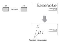
3 Rotate the dial to select a base note from C, C#, D, E♭, E, F, F#, G, A♭, A, B♭ and B. The default setting is "C."
