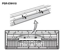
3 Insert the six new batteries, putting them in the correct direction according to the illustration.
